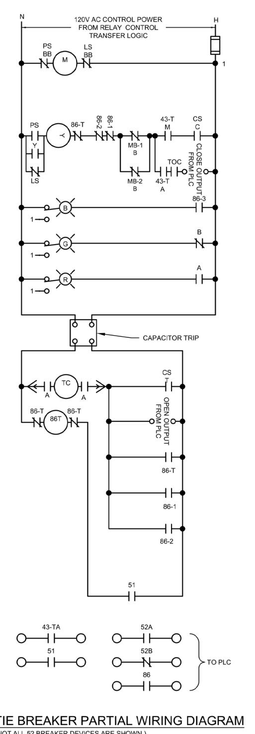
TIE BREAKER PARTIAL WIRING DIAGRAM (NOT ALL 52 BREAKER DEVICES ARE SHOWN.)
