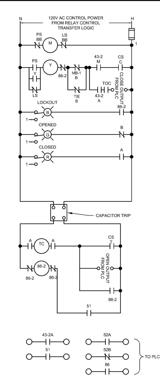
MAIN BREAKER MB-2 PARTIAL WIRING DIAGRAM (NOT ALL 52 BREAKER DEVICES ARE SHOWN.)
